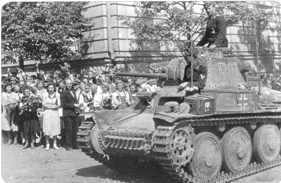
A Pz.Bef.Wg.38(t) drives past a cheering crowd in a Baltic state in 1941. As a command tank, the radio operator's ball mounted M.G.37(t) was removed and plated over and extra radio equipment installed - hence the extra antenna. The 3.7cm Kw.K was also removed and replaced with a fixed dummy gun which has an external 'mantlet' clearly seen here. L.Archer
