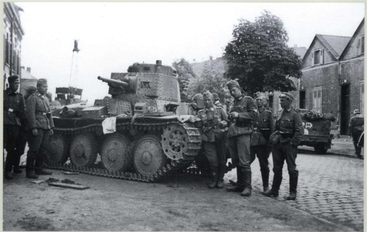
*A Pz 38(t) Ausf B in Luxembourg. The rhomboid-shaped item with holes in it is not an external fitting but an ammunition bin for its main gun, and must have been removed while some work was carried out inside. The divisions between its grey and brown camouflage colours can be seen on the turret and hull front.*
