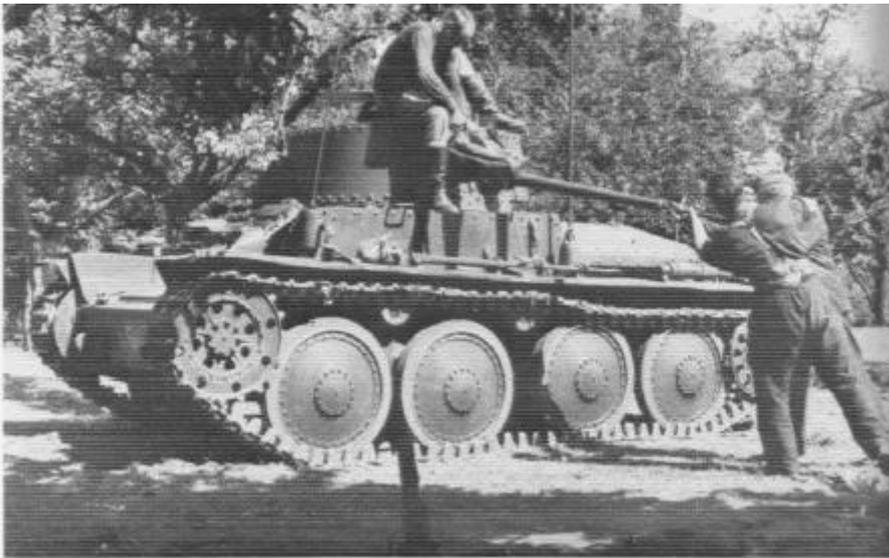
A PzBefW 38(t) ausf A with a Czech whip aerial and a German rod aerial, France 1940. The hull machine gun position has been deleted to make room for the additional radio equipment. Note the stub mount for the Czech tubular "battle" antenna (seen protruding from the front radio antenna mount), and the new Notek blackout light retrofitted to this tank. (Bundesarchiv)
