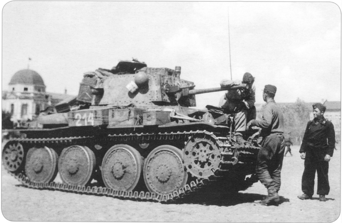
A Pz.Kpfw.38(t) Ausf.G on campaign. It does not carry a national insignia, just the tactical number '214' on a stowage bin attached to the fender. Other stowage bins adorn the fender - all held in place with what looks like string. A 'jerry can' sits in a rack on the turret side, another on the engine deck. A helmet and a mess tin hang from the turret side. L.Archer
