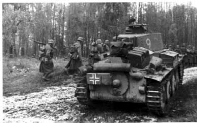
This Page: A Panzerkampfwagen 38 (t) Ausf.S, identified by two rows of five bolts on the front extension of the turret side, did not have increased armor protection on the turret sides and rear or on the superstructure/hull sides. (BA 213/267/12 & 13)
