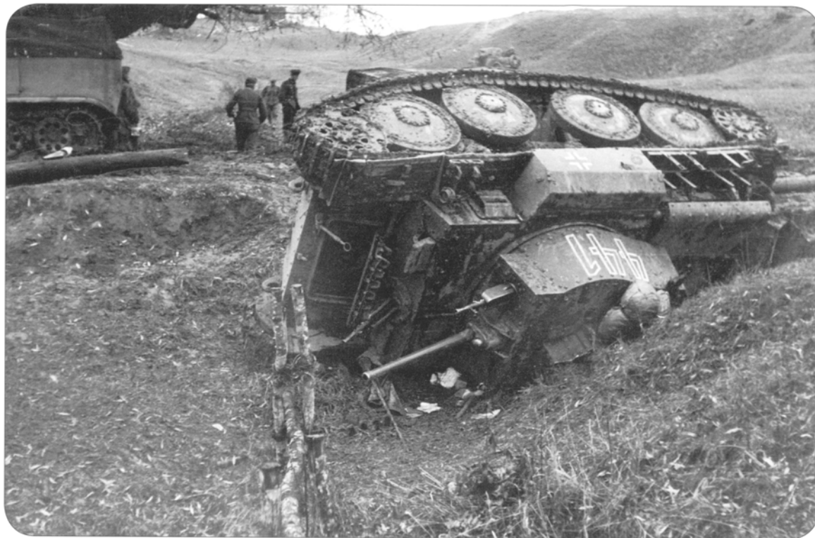
The Pz.Kpfw.38(t) Ausf.E assigned to the platoon leader of the 4.Zug in 4./Kp./II.Abt./Pz.Rgt.27, 19.Panzer-Division has turned turtle into a ditch. The stowage bin on the track guard either side of the fighting compartment, is a feature of vehicles of this unit, as are the 'jerry can' racks on the rear track guards and the two spare track links on the front. L.Archer
