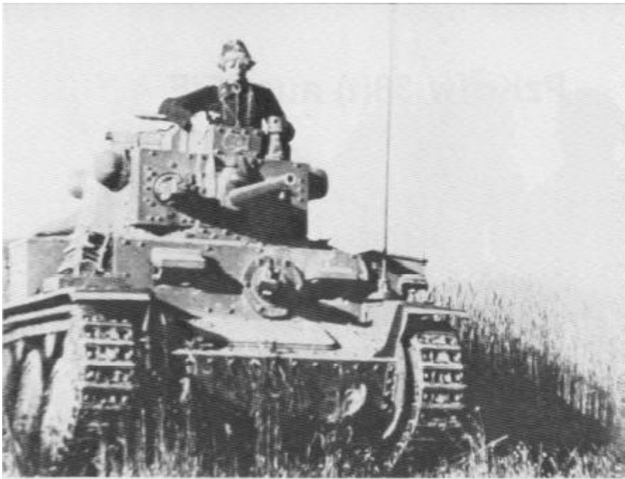
A PzKpfw 38(t) ausf E of the 7th Panzer Division, Russia 1941. Note the driver's straight plate, German type aerial and a Notek light. (Doyle via author)
