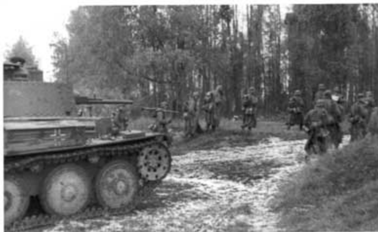
This Page: A Panzerkampfwagen 38 (t) Ausf.S, identified by two rows of five bolts on the front extension of the turret side, did not have increased armor protection on the turret sides and rear or on the superstructure/hull sides. (BA 213/267/12 & 13)
