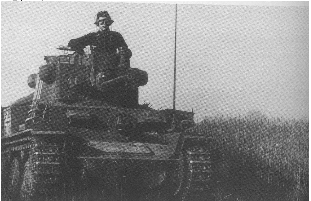
A PzKpfw 38(t) ausf E of the 7th Panzer Division, Russia 1941. Note the driver's straight plate, German type aerial and a Notek light. (Doyle via author)
