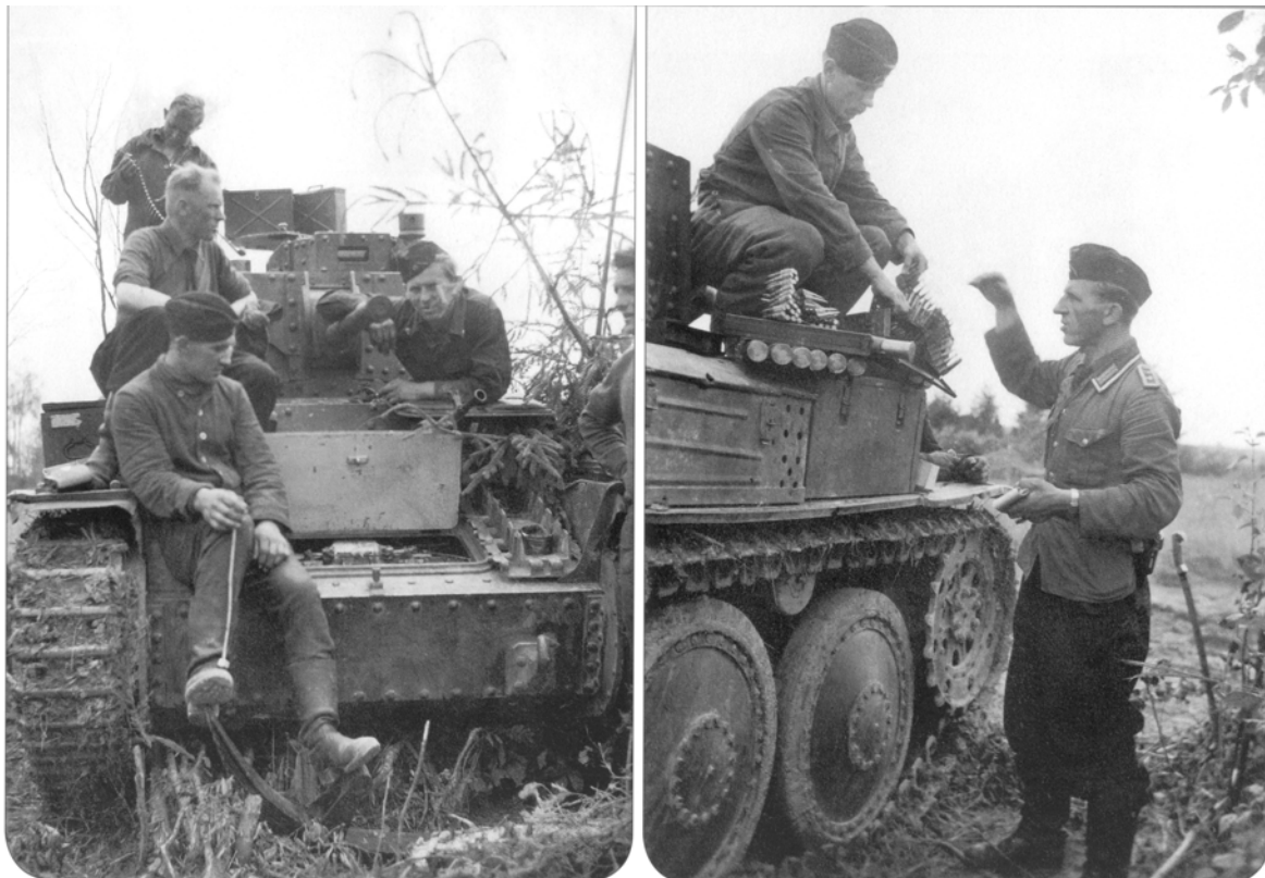
Two shots of a PzKpfw.38(t) Ausf.E or F loading ammunition. In the left picture, with the front steering brake hatch open, we can see that it is painted in RAL 7009 (Hellgrau). The crewman standing in the background is checking the belts of 7.92mm M.G.37(t) ammunition. A total of
